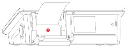
3 After printing, tear the paper upwards.
